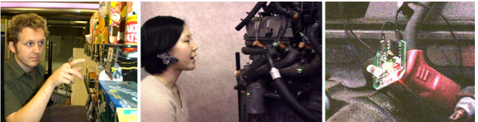
Fig. 1. A user pointing with the finger-worn ring (left), another user wearing the Bluetooth earpiece and interacting with the Engine-Info application (middle), and a close-up of a spark plug-mounted transponder blinking to visually point out the physical object being spoken by the system (right)
