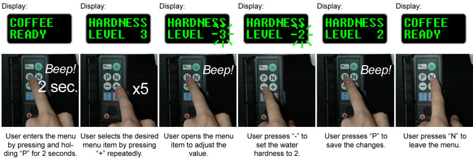
Fig. 3. Example of traditional task solving. At one point, study participants were asked to change the level of water hardness in the coffee maker. The above pictured steps usually required an extensive study of the printed manual.
