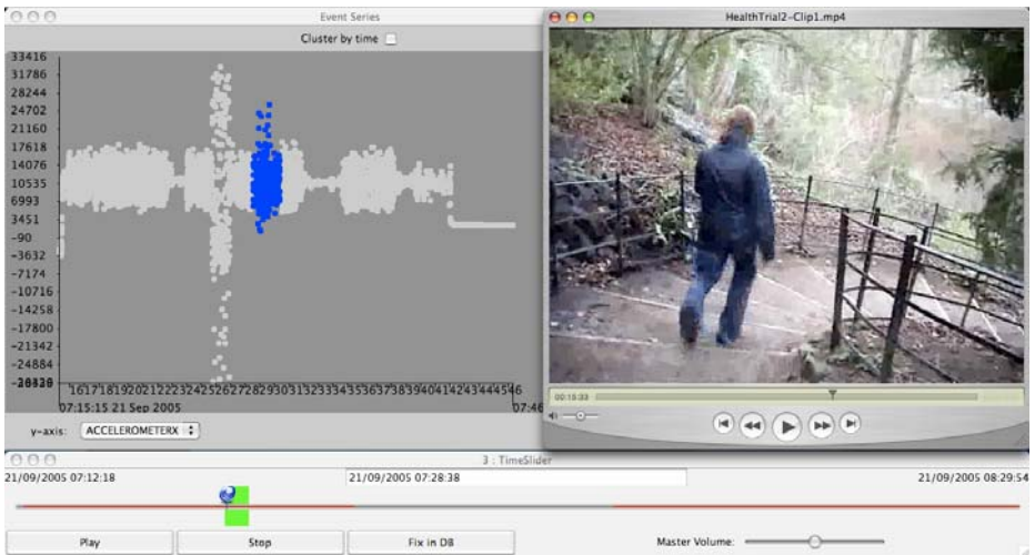
Fig. 1. A simple case of analysing heterogeneous data in Replayer. The analyst has selected a period of time (colouring the selection blue) in graphed accelerometer logs (top left), which triggers Replayer to highlight in green the corresponding section of the video timeline (bottom) and to cue the video of that section (top right). (Colours mentioned here and in other parts of the paper refer to images available in the digital version of this paper).
