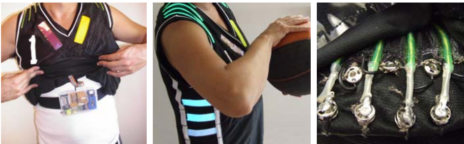
Fig. 4. The wearable computer box attached to athlete's body by harness under the jersey (left); wearable display jersey during use (middle); attachment of displays beneath jersey surface using conductive thread and conductive quick-snap studs for easy detachment (right)
