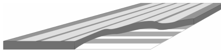
Fig. 1. The leads run in parallel across the foam and form capacitors at their crossover points
