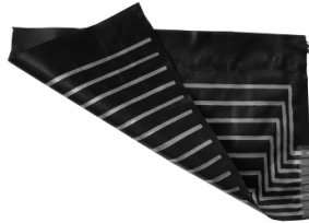
Fig. 3. Conductive silver leads run in parallel across the flexible polyolefin foam to form the 96 sensors. When multiplexed, the leads on different sides of the foam form the capacitive elements.
