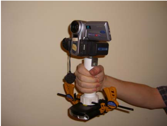
Fig. 5. The camera mount used in the trial. A PDA logging GPS locations, bearings and motion is attached to the base of the mount at a sufficient distance from the camera to be isolated from its magnetic effects.
