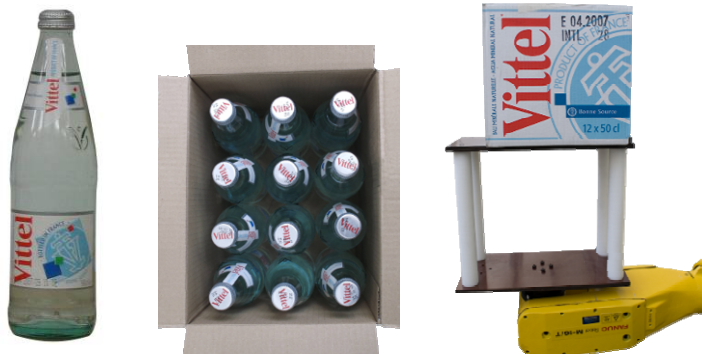
Fig. 11. A photo of one of the 50cl Vittel bottles (left), the inside of the box of Vittel under test, and robot end-effector mounting details for the box
