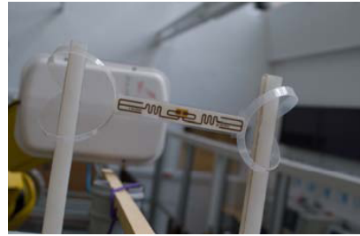
Fig. 8. The custom tag holder allows the RFID tag to be pressed against an object as if it were actually stuck down. Two compliant ‘fingers’ are made from loops of 9x.75mm polyethylene (to the left and right of the tag) and are attached to the robot end-effector using a fairly RF-transparent material. An RFID reader antenna can be seen in the background.
